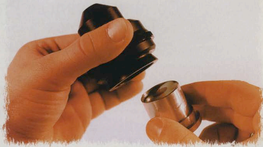
Figure 5. We use a custom-machined metal jig to place our filters in the substage condenser, but homemade jigs from plastic will work as well.
